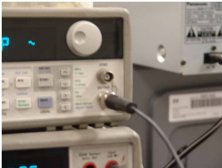
Figure 2. Make sure you use BLACK BNC input cables. Connect them to the OUTPUT terminal as shown above. Do not use the SYNC connector
